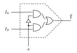
In order to scale this up to larger multiplexers, we need a different method because the standard sum of products method is too inefficient.
