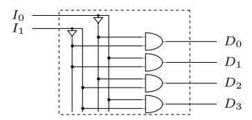
Note that we can only make n to  $2^n$  decoders: The number of outputs must always be a power of two.
