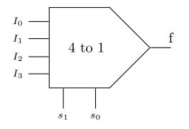
$\begin{array}{ll} \mathrm{If}\;s_1s_0=(00)_2\implies f=I_0.\\ \mathrm{If}\;s_1s_0=(01)_2\implies f=I_1.\\ \mathrm{If}\;s_1s_0=(10)_2\implies f=I_2.\\ \mathrm{If}\;s_1s_0=(11)_2\implies f=I_3. \end{array}$
