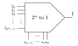
$\begin{array}{l} \text{If } s_{n-1}...s_1s_0 = (00...0)_2 = (0)_{10} \implies f = I_0.\\ \text{If } s_{n-1}...s_1s_0 = (00...1)_2 = (1)_{10} \implies f = I_1. \text{ And so on...}\\ \text{If } s_{n-1}...s_1s_0 = (11...1)_2 = (2^n - 1)_{10} \implies f = I_{2^n - 1}. \end{array}$
